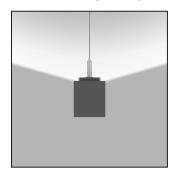
Wide smooth indirect batwing distribution enables greater row spacing while maintaining ideal ceiling uniformity. Find the flexibility you need, or reduce fixture count without creating harsh contrast.
