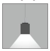
Soft uniform illumination in a symmetrical 2"x2" aperture with a 45° cutoff angle. Unified Glare Ratings (UGR) of less than 13 and as low as 0 in some configurations.
